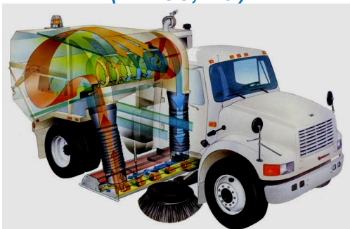
Figure 17. Regenerative Air Cleaner (TYMCO, Inc.)
