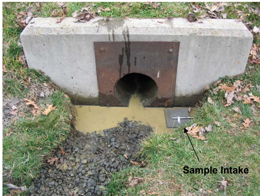
Figure 2: Outlet Monitoring at University Dry Detention Basin.
