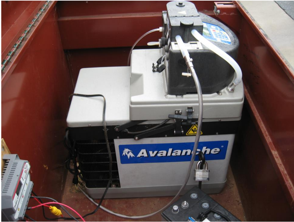
Fig 3.1 ISCO Avalanche Model 6712 sampler
