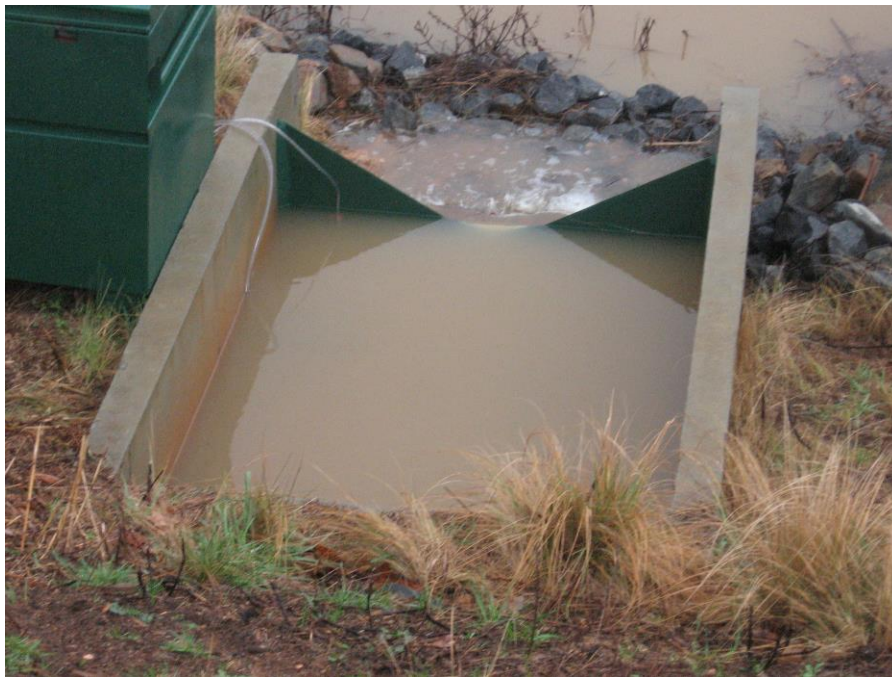
Fig 5.1 120 degree V-notch weir measuring flow from a parking lot.
