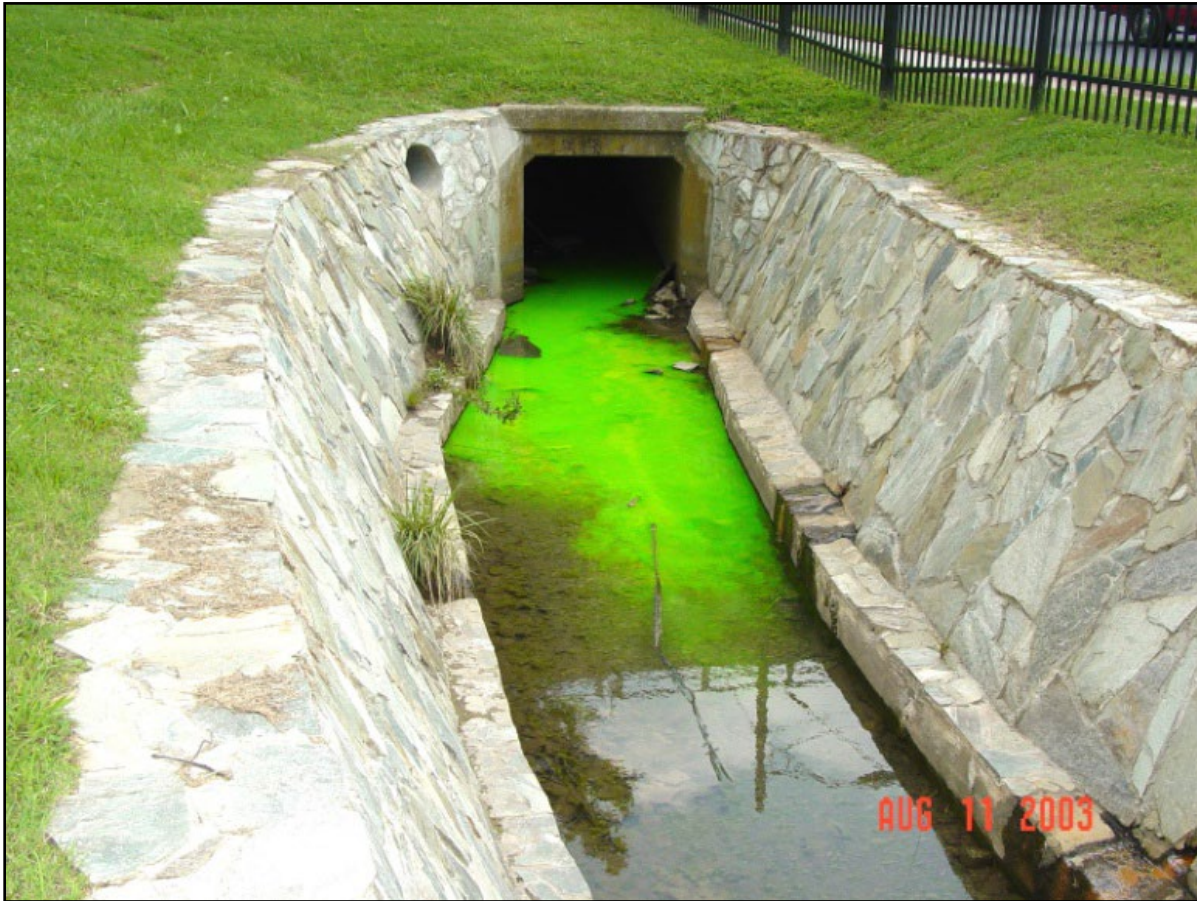
Figure 4-3: A successful dye test reveals a discharge of sewage from apartments.
