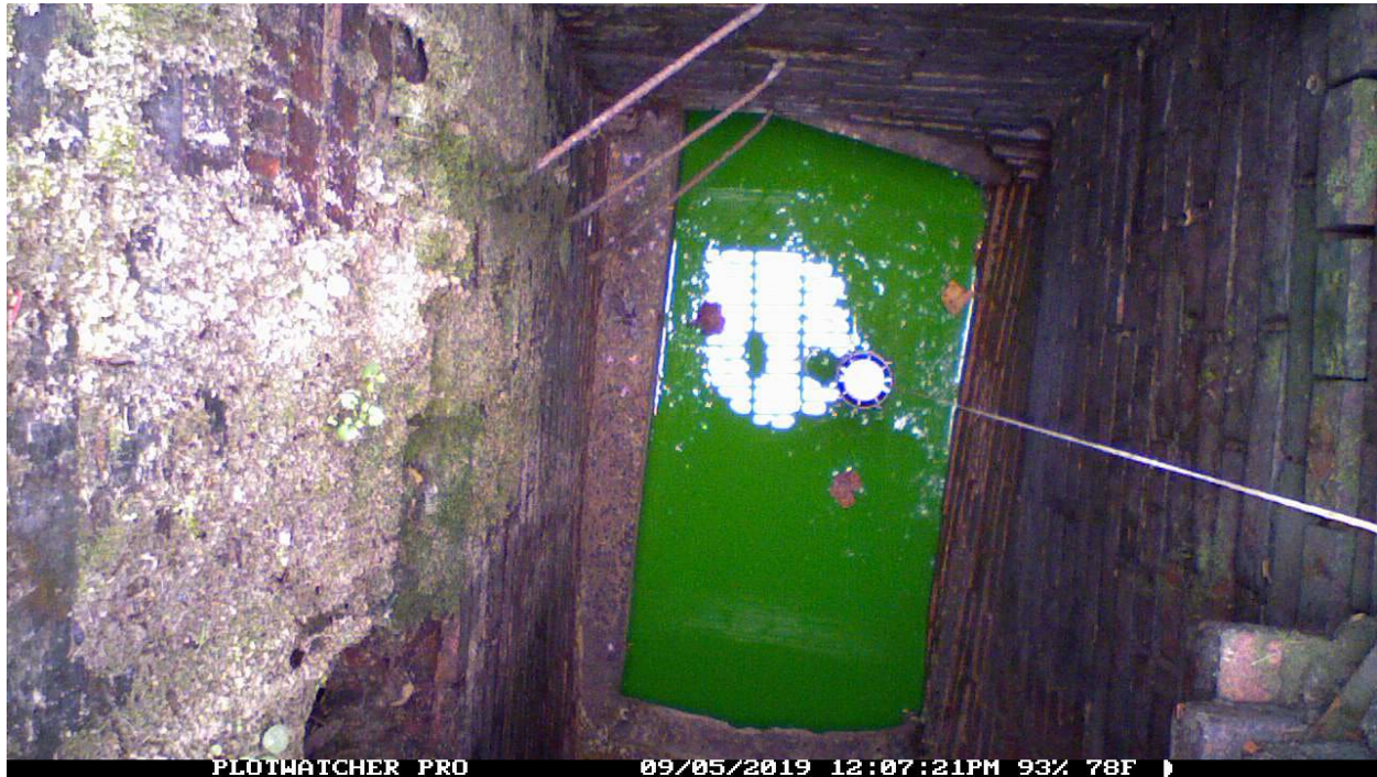
Figure 4-7: Illicit connection verified using a dye test and stationary camera setup in a drop inlet to monitor the progression of dye.
