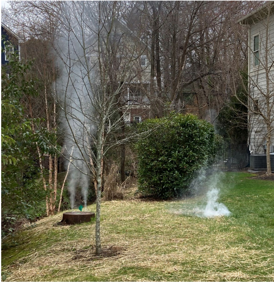
Figure 4-4: Smoke exiting a manhole while conducting a smoke test in the area.
