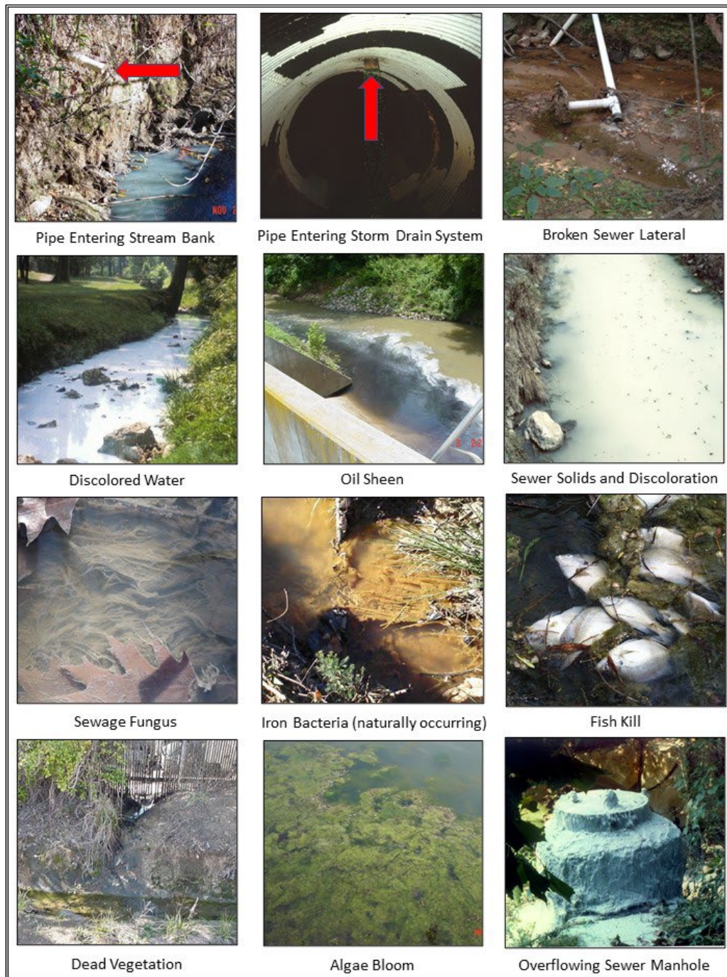
Figure 3-1: Field observations indicating an illicit discharge.
