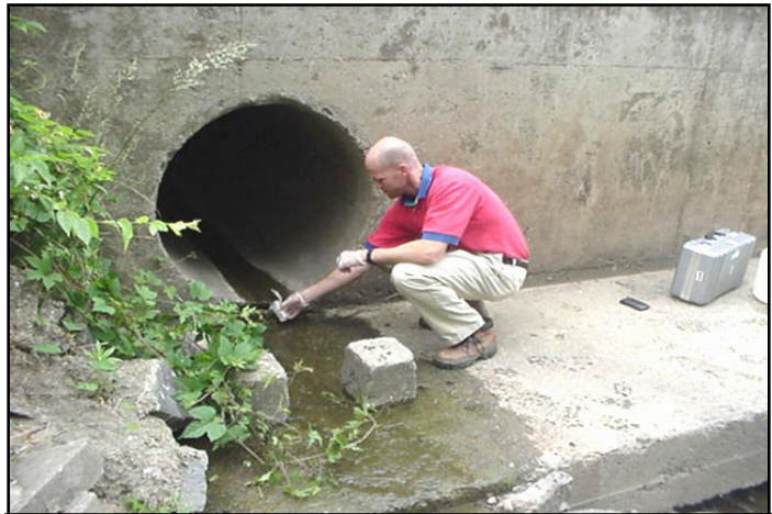
Figure 3-2: Dry weather flow sampling by CMSWS staff during stream walk.
