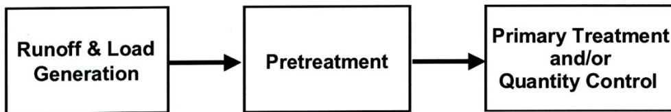
Generalized Storm Water Treatment Train
