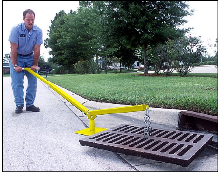
Storm drain grate lifter - allows one person to safely remove and replace a heavy grate.
