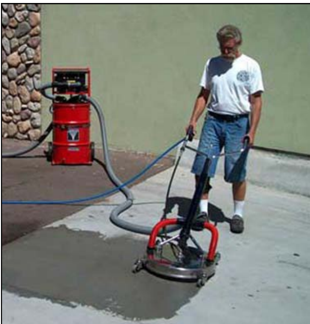
This all-in-one unit vacuums the wash water as it cleans the surface.
