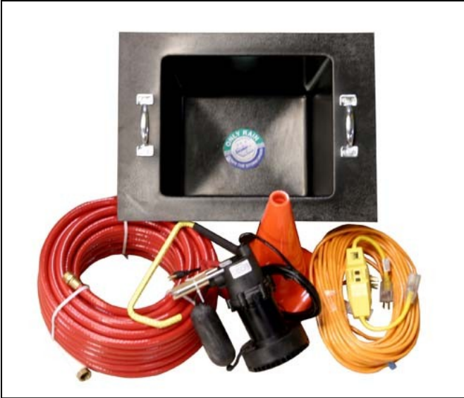
Storm drain basin insert - fits into a storm drain catch basin and collects wash water as it enters. Insert a sump pump in the basin with a hose connected to a tank to collect water.
