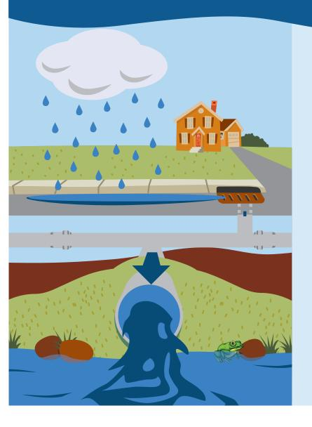
Stormwater goes directly to our creeks and lakes without treatment. Pollution that washes away with rain and enters storm drains is called stormwater pollution.
