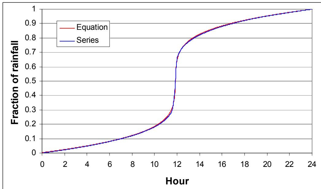
Figure 1. SCS 24-hour Type II Storm – Comparison of Tabular Values to Fitted Equation
