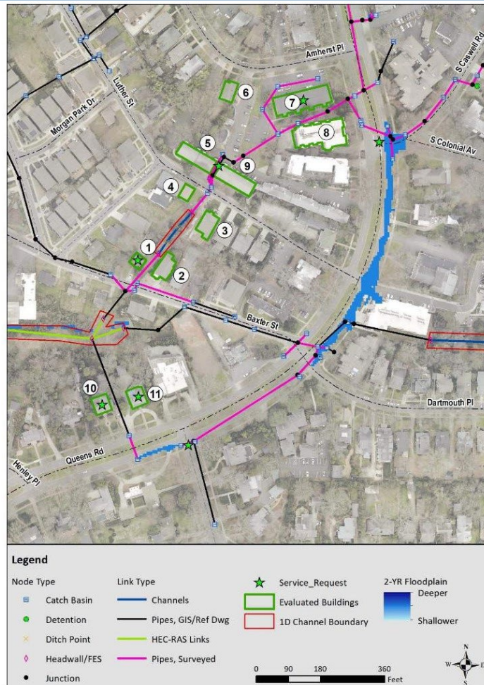
Figure EC- 23: Inundation Map of Detailed Study Area, 2-yr 6-hr Storm, Existing Conditions
