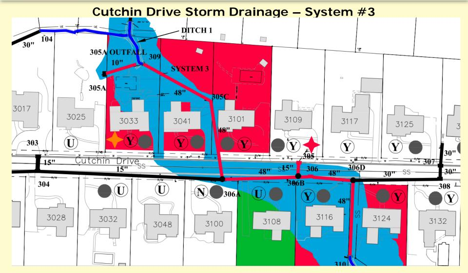
•System #3 - Additional inlets needed & system undersized for 10yr storm event causing flooding at 6 residences.
