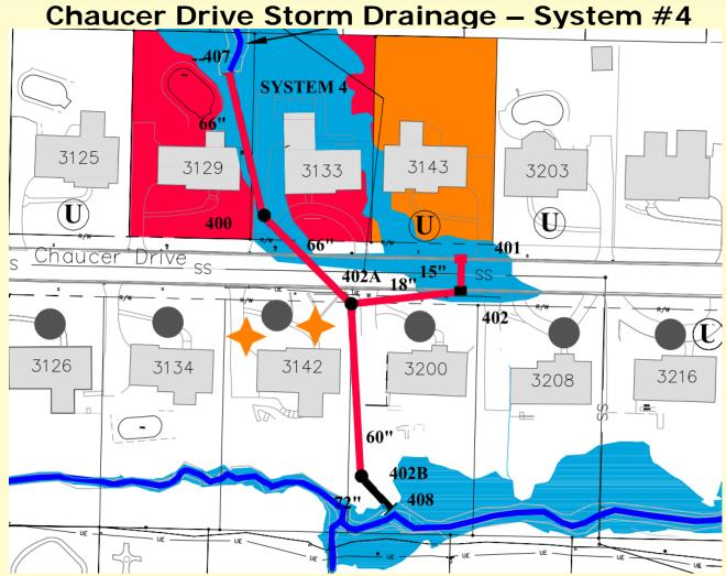
•System #4 - Additional inlets needed & system undersized for 25yr storm event causing flooding at 3 residences.
