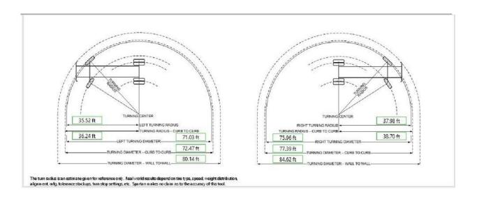
End User Name Charlotte Fire Department 0100-012 Gladiator Chassis Model Wheelbase 250.00 in **Bumper Extension** 6.00 in 104.40 in Bumper Width Left hand outside tire turn angle 33.50 deg Right hand outside tire turn angle 31.00 deg Left hand Curb-to-Curb turning radius 36.24 ft, 11.04 m Right hand Curb-to-Curb turning radius 38.70 ft, 11.79 m Left hand Wall-to-Wall turning radius 40.07 ft, 12.21 m Right hand Wall-to-Wall turning radius 42.31 ft, 12.90 m
