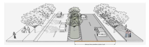
**b. Morris Estate Drive:** The future location of the back of curb is to be placed at 24-feet from the roadway centerline to accommodate the cross section of a 2+ avenue with bike lanes. This future back of curb location will vary at the intersection with the addition of a turn-lane and other intersection geometry features.
