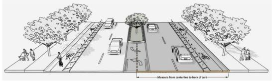
a. Limelight Lane: The future location of the back of curb and gutter is minimum 17.5' from roadway centerline following CLDSM U-03A1 detail.
