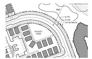
6. Outstanding Comment from 8/28/25: Revise site plan and conditional note(s) to commit to adding conditional note to meet all minimum roadway requirements including but not limited to vertical and horizontal roadway alignment and intersection angle requirements. (i.e. appears to be a reverse curve over Banner Ridge, would need to verify that it meets the minimum requirements and the proposed southwest intersection internal to the site must have a minimum intersection angle of 75 degrees)
