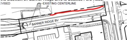
Outstanding Comment from 8/28/25: Revise site plan and conditional note(s) by adding pedestrian ramps to the intersections within the proposed development. You may need to adjust some of the on street parking stalls to accommodate.
