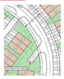
8. Revise site plan to create a minimum 10 foot separation from the curb return to the property line for the access along Plaza Road.
