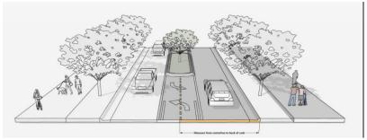
b. Neal Road: Location of future curb and gutter is to be 19 feet from roadway centerline to back of curb. This location does not include additional turn lanes.
