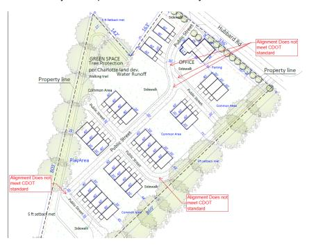
8. Revise site plan and conditional notes to remove the southernmost site access to Hubbard Road due to Access restriction requirements per Charlotte Streets Manual and not meeting intersection spacing requirements.
