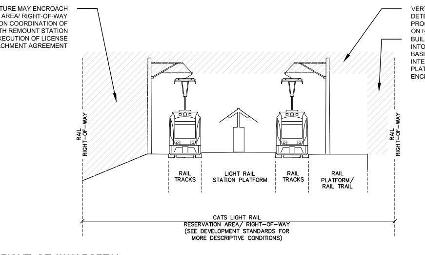
VERTICAL CLEARANCE TO BE DETERMINED IN LAND DEVELOPMENT PROCESS IN COORDINATION WITH CATS ON REVIEW OF ADVANCING DESIGN BUILDING STRUCTURE MAY ENCROACH INTO RESERVATION AREA/ RIGHT-OF-WAY BASED ON COORDINATION OF INTERACTION WITH REMOUNT STATION PLATFORM AND EXECUTION OF LICENSE ENCROACHMENT AGREEMENT
