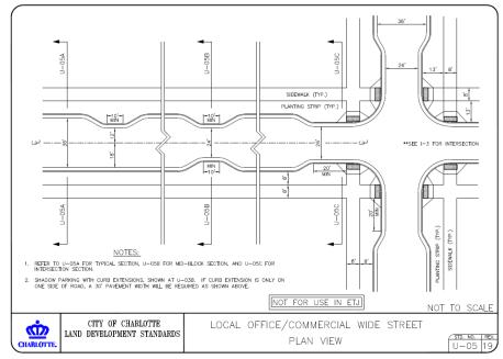
NOTE: Additional distance from center line to back of curb may be required in locations where a median is present or around intersections and interchanges.
