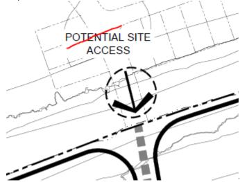
9. Outstanding Issue 8/24/23: Remove this intersection, and ensure all future horizontal curves meet the minimum CDOT standard of 150' radius.
