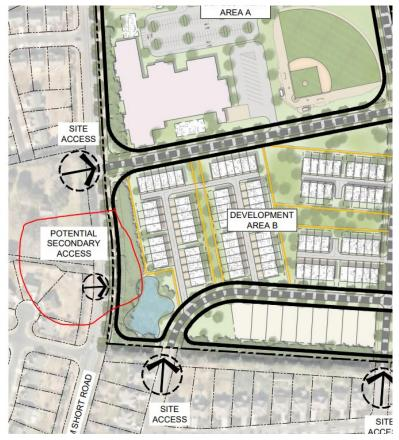
b. A POTENTIAL SECONDARY ACCESS FROM TOM SHORT RD. TO DEVELOPMENT AREA B IS PROPOSED. THIS SECONDARY ACCESS IS SUBJECT TO FURTHER REVIEW AND APPROVAL BY CDOT AND NCDOT. THE SPECIFIC DESIGN OF THE PROPOSED ACCESS TO TOM SHORT RD. WILL BE DETERMINED DURING THE LAND DEVELOPMENT APPROVAL PROCESS. THE PETITIONER RESERVES THE RIGHT TO NOT MAKE THIS SECONDARY CONNECTION IF ADDITIONAL RIGHT-OF-WAY OR UTILITY RELOCATIONS FOR THIS CONNECTION ARE REQUIRED.
