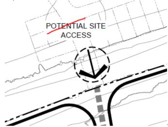
7. Outstanding Issue 8/24/23: Remove this intersection, and ensure all future horizontal curves meet the minimum CDOT standard of 150' radius.
