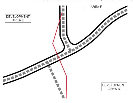
8. Outstanding Issue 8/24/23: The horizontal curves pictured below need to have a minimum 50' separation to meet minimum CDOT standard.
