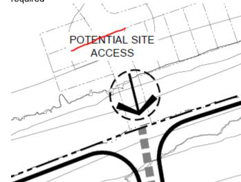
6. Outstanding Issue 8/24/23: Remove this intersection, and ensure all future horizontal curves meet the minimum CDOT standard of 150' radius.
