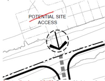
7. Outstanding Issue 8/24/23: Remove this intersection, and ensure all future horizontal curves meet the minimum CDOT standard of 150' radius.
