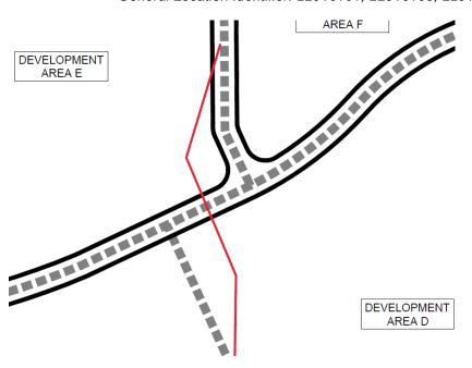
9. Outstanding Issue 8/24/23: The horizontal curves pictured below need to have a minimum 50' separation to meet minimum CDOT standard.
