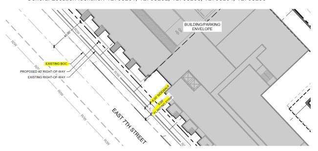
14. New Comment 9-20-23: Revise site plan to eliminate encroachment of building and building entrances into the right-of-way.
