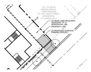
Clarifying Comment 9-20-23: Remove the additional parking spaces on Clement and Lamar Ave. Access to parking spaces is not allowed over a streetscape. This access would be considered a driveway and would be required to meet minimum driveway standards including geometric design, spacing, and internal stem requirements.
