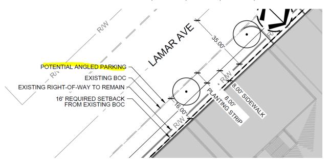
16. New Comment 11-27-23 – The sidewalk + 2' behind the sidewalk must be located within the ROW or sidewalk utility easement (SUE). If the existing ROW is remaining on Lamar and Clement Ave, then add SUE to encapsulate sidewalk + 2'
