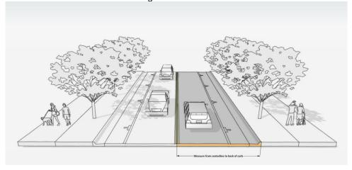
NOTE: Additional distance from center line to back of curb may be required in locations where a median is present or around intersections and interchanges.
