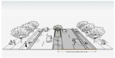
b. **Myrtle Avenue:** Location of curb and gutter to be moved to 20.5 feet from roadway centerline to accommodate the local commercial wide street typical section with on street parking (CLDSM U-05 Series).
