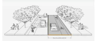
b. Yorkmont Road: Location of curb and gutter to be installed 24 feet from roadway centerline to the back of curb to accommodate the Charlotte Streets Map with a roadway typical section of a 2+ avenue with bike lanes, 8 foot sidewalk and 8 foot planting strip.
