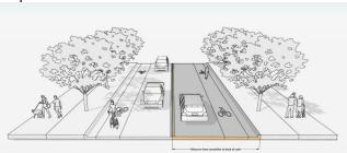
b. **Yorkmont Road:** Location of curb and gutter to be installed 24 feet from roadway centerline to the back of curb to accommodate the Charlotte Streets Map with a roadway typical section of a 2+ avenue with bike lanes, 8-foot sidewalk and 8-foot planting strip.
