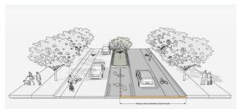
NOTE: Additional distance from center line to back of curb may be required in locations where a median is present or around intersections and interchanges.
