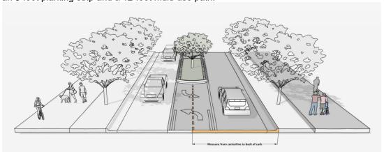
NOTE: Additional distance from center line to back of curb may be required in locations where a median is present or around intersections and interchanges.
