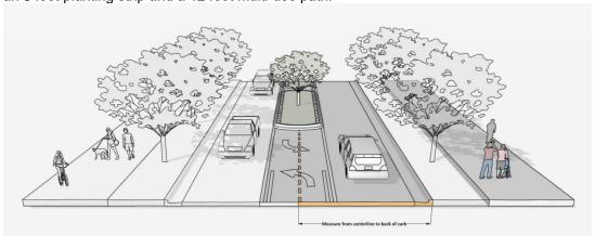
NOTE: Additional distance from center line to back of curb may be required in locations where a median is present or around intersections and interchanges.
