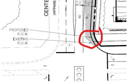
7. Revise site plan and conditional note(s) to commit to construct an 8-foot planting strip, and 6-foot sidewalk on Centergrove Lane and Lakebrook Road per Chapter 19. The site plan shall label and dimension both items from the back of curb and gutter or edge of pavement. Install curb and gutter per CLDM U-06 for local industrial wide typical section.
