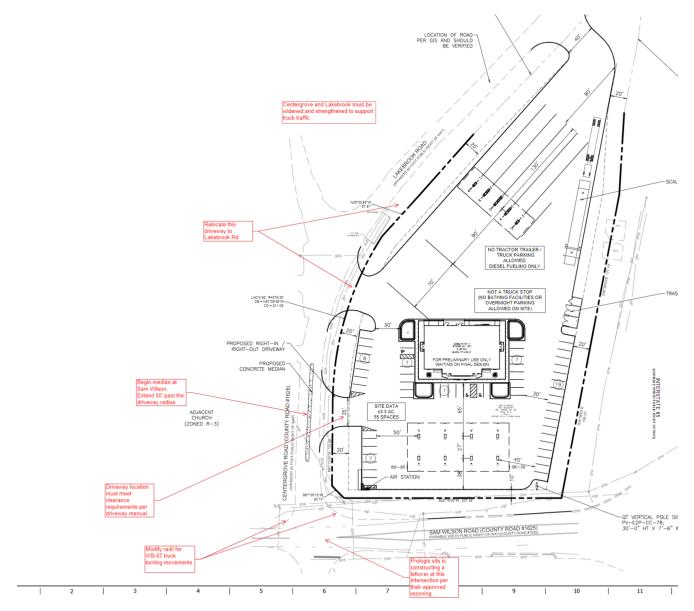
4. Revise site plan and conditional note(s) to commit to dedicate 35 feet of right of way from the road centerline on Sam Wilson Road. The site plan shall label and dimension the right-of-way from the road centerline.
