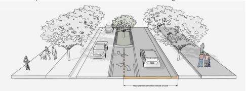
**Steele Creek Road:** Location of curb and gutter to be installed a minimum of 33 feet from roadway centerline to accommodate the Charlotte Streets Map with a roadway typical section of a 4+ Avenue. Coordination with U-5766B project is required to confirm future back of curb location. Additional distance from center line to back of curb may be required in locations where a median is present or around intersections and interchanges.
