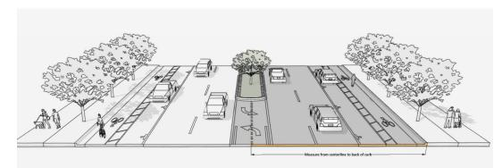
b. Clanton Road: Location of curb and gutter to be moved a minimum of 27 feet from roadway centerline to accommodate the Charlotte Streets Map with a roadway typical section of a 2+ Avenue with Buffered/Separated Bike Lanes.
