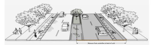
NOTE: Additional distance from center line to back of curb may be required in locations where a median is present or around intersections and interchanges.
