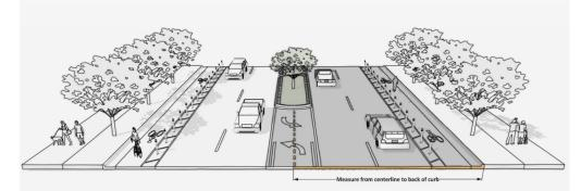
NOTE: Additional distance from center line to back of curb may be required in locations where a median is present or around intersections and interchanges.
