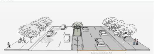
NOTE: Additional distance from center line to back of curb may be required in locations where a median is present or around intersections and interchanges.
