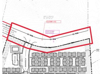
6. CDOT REQUEST 03-23-23: CDOT request that Legranger is revised to meet CLDSM U-02 between the sites frontage and the proposed site access to plan west. If this section is not complete the western most site access location shall be required to be restricted to emergency vehicular entrance only. This entrance shall be gated with a knox box.
