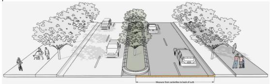
b. Parkside Crossing: Location of the future curb and gutter to be installed at 17.5 feet from roadway centerline to accommodate the Charlotte Streets Map roadway typical section of collector street per CLDSM U-07. The future curb and gutter should be shown on the plan
