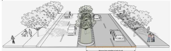
b. **Parkside Crossing:** Location of the future curb and gutter to be installed at 17.5 feet from roadway centerline to accommodate the Charlotte Streets Map roadway typical section of collector street per CLDSM U-07. The future curb and gutter should be shown on the plan and dimensioned from the centerline.
