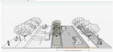
b. **Creston Road:** Location of curb and gutter to be installed at 17.5 feet from roadway centerline in accordance with the Local Residential Wide typical section (CLDSM U-03).
