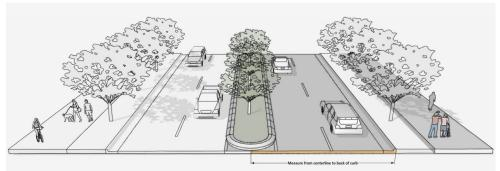
Label and dimension the curb and gutter from the centerline for each road on the site plan.
