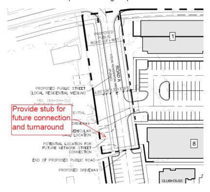
8. Revise site plan and conditional note(s) to relocate the proposed gate a minimum of 40ft from the right of way on Road A
