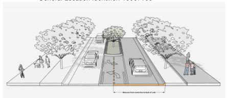
NOTE: Additional distance from center line to back of curb may be required in locations where a median is present or around intersections and interchanges.
