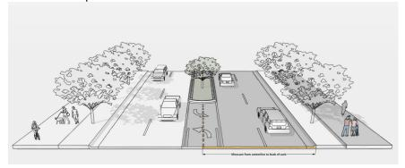
b. **Sledge Road:** Location of curb and gutter to be moved to 19 feet from roadway centerline to accommodate the Charlotte Streets Map with a roadway typical section of a two plus lane avenue with shared use path.
