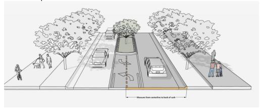
Thomas Road: Location of curb and gutter to be located 17.5 feet from roadway centerline to accommodate the Charlotte Streets Map with a roadway typical section of a two plus lane avenue with sidewalk. The location of curb and gutter is in accordance with CLDSM U-06 for local collector.
