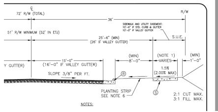
NOTE: Additional distance from center line to back of curb may be required in locations where a median is present or around intersections and interchanges.
