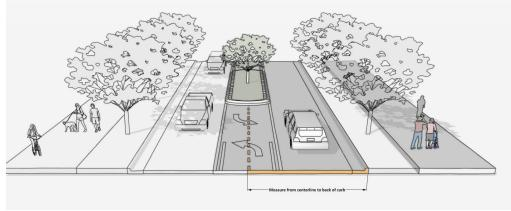
**Thomas Road:** Location of curb and gutter to be located 17.5 feet from roadway centerline to accommodate the Charlotte Streets Map with a roadway typical section of a two plus lane avenue with sidewalk. The location of curb and gutter is in accordance with CLDSM U-06 for local collector.
