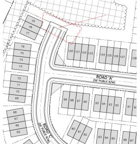
10. Revise site plan to provide a minimum internal stem length of 50' between radius returns along Road
