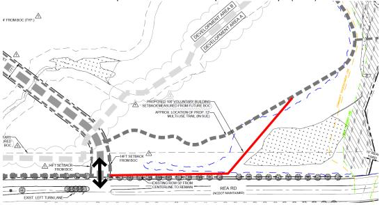
4. Revise site plan and conditional note(s) to install the new public street as a local collector per CLDSM U-06.
