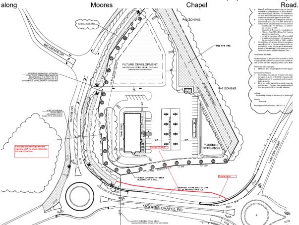
5. Outstanding Comment Revise site plan and conditional notes to provide curb and gutter along the public roads that front the proposed tree save parcel. The minimum distance to the back of curb and gutter is 19-feet from the centerline of Rhyne Road and 30-feet from the centerline of Moores Chapel Road.
