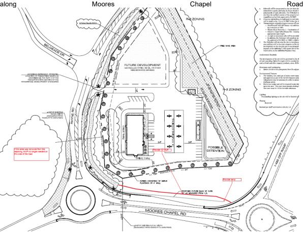
4. Outstanding Comment Revise site plan and conditional notes to provide curb and gutter along the public roads that front the proposed tree save parcel. The minimum distance to the back of curb and gutter is 19-feet from the centerline of Rhyne Road and 30-feet from the centerline of Moores Chapel Road.
