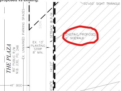
6. Revise site plan and conditional note(s) to show existing western driveway to be removed and curb and gutter to be replace driveway on Commonwealth Avenue.
