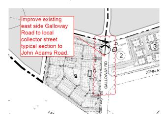
3. Revise site plan and conditional note(s) to commit to the proposed roadway network typical sections and proposed phasing outlined in the Traffic Impact Study. Provide typical sections per CLDSM for all proposed public and private streets. Provide 8-foot sidewalk and 8-foot planting strip on all public streets.
